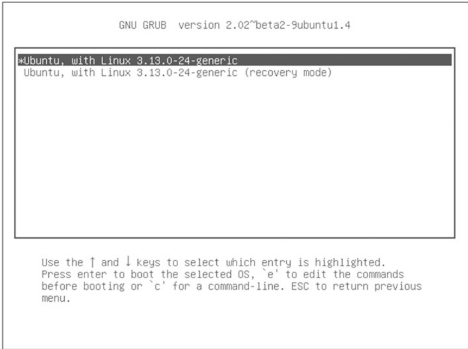
Figure 1-3. A GRUB advanced menu (accessed by selecting “Advanced options” in the main menu window)
